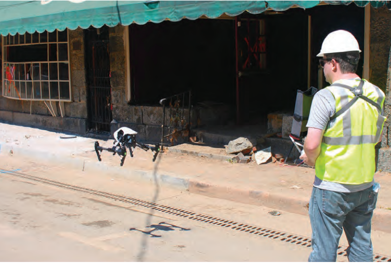
Maryland-based drone specialists Elevated Element completed an aerial survey of Main Street in Ellicott City. The drone accessed many areas unsafe for people.
