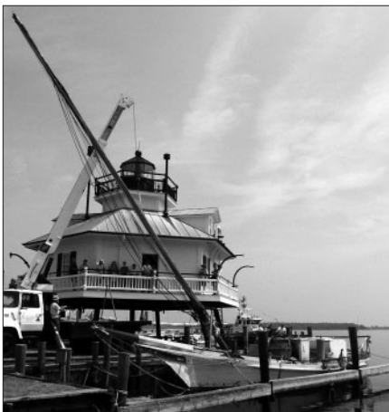
Work on the commercial skipjack Somerset begins with the pulling of its mast. As part of the Save Our Skipjacks Task Force recommendations a restoration program for commercial skipjacks was created at the Chesapeake Bay Maritime Museum.
